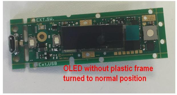
When the user wants to place the display somewhere else in the box/application, instead of plugging the OLED directly to the onboard FPC, a standard 12pin 0.5mm pitch FFC cable can be connected to the board which is then connected to a display carrier board at the other end.
